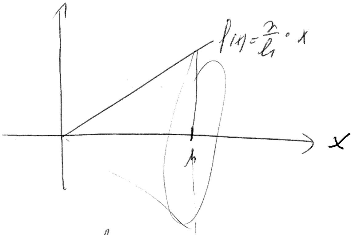
$$V_{\text{Rot}} = \pi \cdot \int_a^b [f(x)]^2 dx$$
